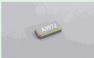
External dimensions: 32 x 15 x 0.9t mm, Max. Frequency tolerance: ±20 × 10 -6 ; operating temperature range: -40 to 125°C
